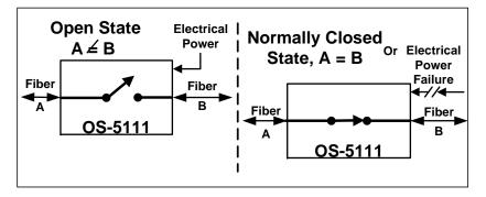
The OS-5111 switch will go into the close state under any of the following conditions:
