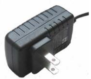
The PS-1205US is a plug-in wall adapter designed to power most Fiber transmission units. The unit converts 115 VAC 60 Hz to 12 volts DC at up to 500 milliamperes. The wire with the white stripe is the positive lead (+), the unmarked wire is the negative lead.
