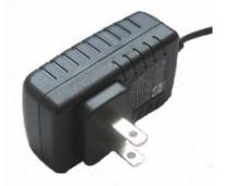
The PS-1205US is a plug-in wall adapter designed to power most Fiber transmission units. The unit converts 115 VAC 60Hz to 12 volts DC at up to 500 milliamperes. The wire with the white stripe is the positive lead (+), the unmarked wire is the negative lead.
