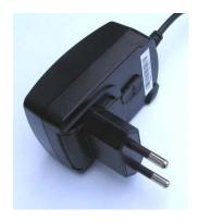
The PS-1208EU is a plug-in wall adapter designed to power most Fiber transmission units. The unit converts 100-240 VAC 50/60Hz to 12 volts DC at up to 800 milliamperes. The wire with the white stripe is the positive lead (+), the unmarked wire is the negative lead.
