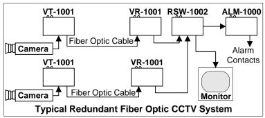
Upon loss of the primary video signal, the RSW-1002 will automatically switch the remaining secondary (backup) video signal to the output as well as activate the front panel alarm "Alm" indicator and ALM-1000 Alarm Sensing Unit if used.
