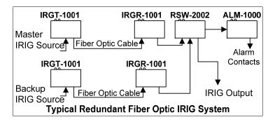
Upon loss of the primary IRIG signal, the RSW-2002 will automatically switch the remaining secondary (backup) IRIG signal to the output as well as activate the front panel alarm indicator and ALM-1000 Alarm Sensing Unit if used.
